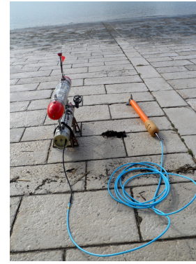
Fig. 8. Magnetic sensor cabling and connection to the Medusa ASV.
